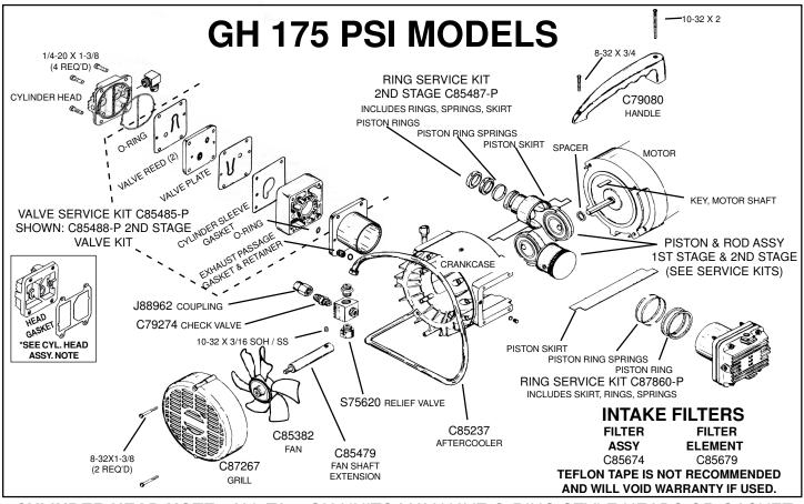
CYLINDER HEAD NOTE: ALL TA & GH UNITS MAY HAVE O-RING STYLE HEADS OR GASKET STYLE HEADS INSTALLED AT FACTORY. THE VALVE SERVICE KIT COVERS BOTH STYLES.
