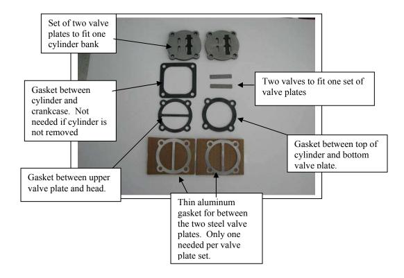
One Valve plate kit and one gasket kit is needed for each cylinder that is being repaired.
